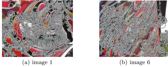
Fig. 1. Harris Laplacian detector applied to the graffiti testset (see Fig. 7(a)) image 1 (a) and image 6 (b). The size of the circles indicates the size (scale) of the kernel with the highest peak.
